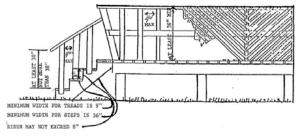
Guardrails shall be located at least 36 inches above the floor.
